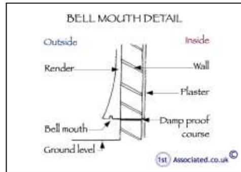
even if there is a damp proof course the render gives the dampness a way to bypass the damp proof course. In such situations you simply need to add a bell-mouth detail to the base of the render at the appropriate level.
