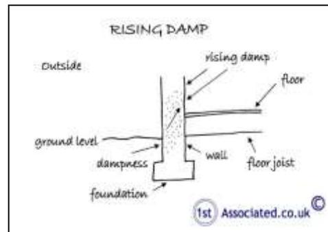
Different types of construction, such as stone construction or where the property sits on a sloping site, may have slightly different readings, but in our experience generally rising damp rises to about a metre.
