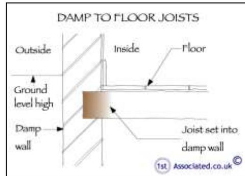
The good Building Surveyor will carry out various tests to see if there is deterioration in this area. Some of the tests can be carried out without opening up the floor, but in older properties we would always recommend that the floor is opened up and each joist is examined. Repair will be on an individual basis.
