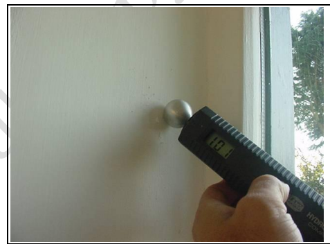
Damp meter reading of 101
