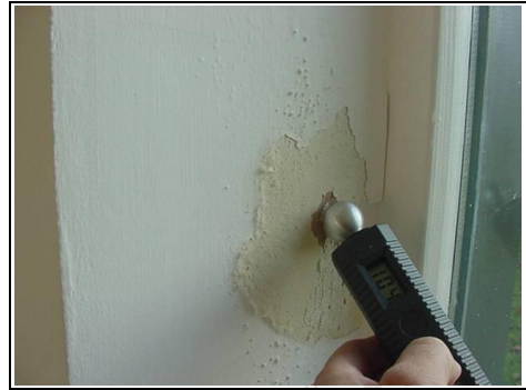
Damp meter reading of 104 on the reveal
