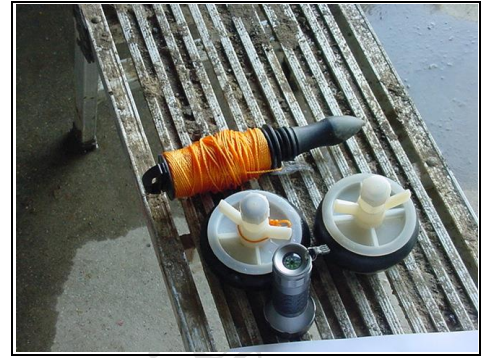
Bungs used for water testing
